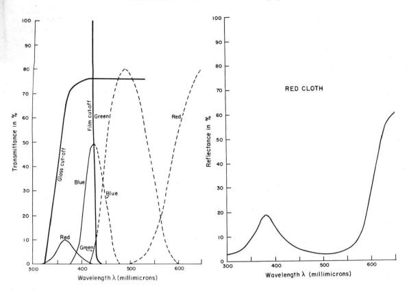
Fig. 1. Transmittance curves for the red, green and blue filters and the lens glass and a curve showing the long wavelength cut-off of the film (film sensitive to all shorter wavelengths).
