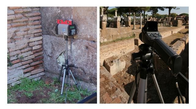
Figure 4: The spectroradiometer Minolta CS-1000A (left). Figure 5: The thermal camera FLYR (right).
