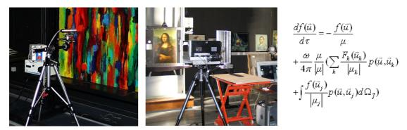
Figure 1: Three means to pursue the colour of masterpieces in the INSP: goniospectrometer in back-scattered configuration (left) [3], multispectral camera of Lumière Technology (middle) [4], and radiative transfer equation RTE (right) [6,7].
