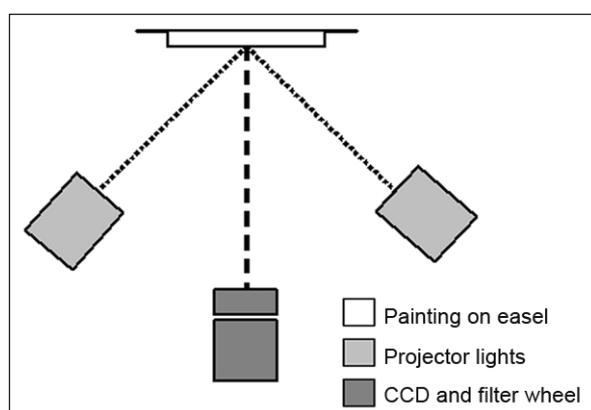
**Figure 4** Hyperspectral imaging system setup, seen from above
