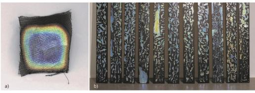
Figure 10: (a) An example of the coffee ring effect in a textile sample coated with nanocellulose that generates structural colour. The effect makes the edge colours transition towards yellow and red. (b) The "Morpho" artwork showing the coffee ring effect being utilised to create patterns for design objects. Edge colours play an important role in the pattern design of the work called Morpho. Artwork: Structural Color Studio (Noora Yau and Konrad Klockars) Photo: Esa Naukkarinen.
