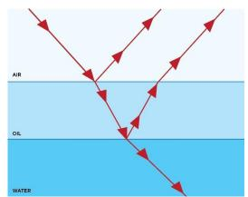
Figure 4: Schematic illustration of thin-film interference, where the red lines represent light rays of a wavelength that experiences constructive interference. Varying the direction of the incoming light beam changes which wavelengths of light experience constructive or destructive interference. This results in the change of colour (iridescence) perceived with the illumination/viewing angle.
