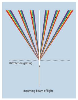
Figure 6: Schematic illustration showing how a diffraction grating splits an incoming light ray (white) into several rays having gradients of wavelengths (colours).
