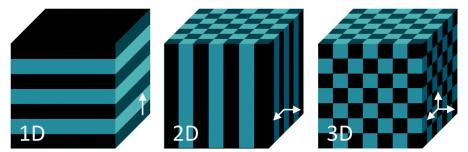
Figure 8: Schematic illustration of photonic crystals with periodicity in 1, 2 or 3 dimensions. Adopted from [67].
