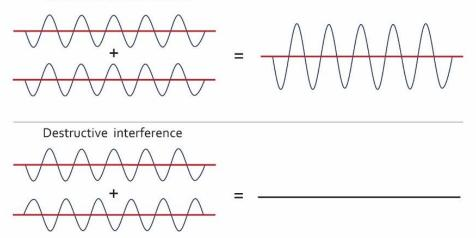
Figure 3: Illustrations explaining constructive and destructive interference in terms of the wave properties of the light beam.
