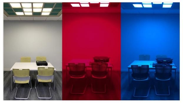
Figure 1: Three coloured-lighting conditions created with a Thouslite LED system. Note that the computer was not in the environments during either the physical or VR experiments.
