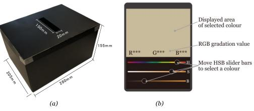
Figure 2: (left) Black box and (right) Colour chart software on display.
