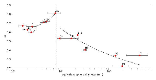
Figure 4: Hue against the equivalent sphere diameter deduced from SEM experiments. The hue is increasing for very small particles until a critical diameter (~80 nm, dot line) where the trend is reversed.
