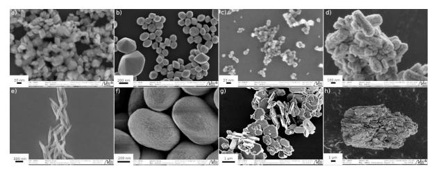
Figure 2: SEM images of the different hematite powders. a) Crystals of samples 1, 1<sub>2</sub>, 2, 5 and 6 show pretty similar morphology: same diamond shape and close sizes. Only 1 is shown here. b) Sample 3 presents two bipyramid shaped crystal populations different in size. c) Sample 4 is composed of very small spherical particles.
