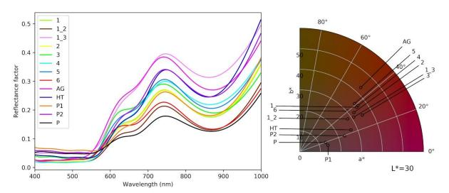
Figure 3: Reflectance spectra of the samples (left), calibrated by a Spectralon<sup>®</sup>, and position of the corresponding colours in the CIE L\*a\*b\* diagram for L\*=30 (right).
