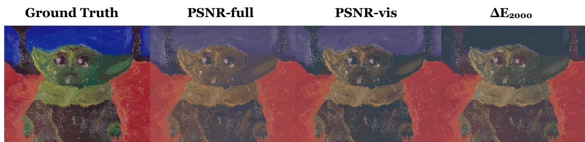
Figure 3: Renderings in sRGB from the pigment mapping inverting the hybrid Yule-Nielsen model. The different cost functions vary from left to right: ground truth, optimisation utilising the full range of wavelengths (400-1000nm), optimisation for PSNR only in the visible range, optimisation for \Delta E_{2000} .
