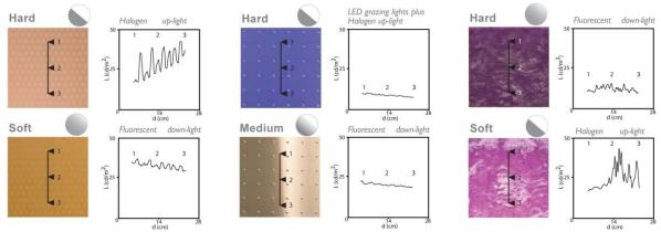
Figure 3: Photographs and measured luminance profiles for three samples lit by fluorescent and halogen sources. The numbers describe three positions along the measured profiles. The disk symbol indicates light diffuseness.
