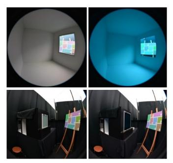
Figure 7: Above: Fish-eye photographs of scale models with ET glass (left) and EC-coloured glass (right). Below: Exterior view of scale models with ET glass (left) and EC-coloured glass (right).
