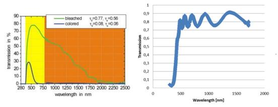
Figure 2: Light transmission data for EC glazing from GESIMAT (left) and for PC glazing from IFE (right).
