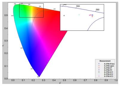
Figure 15: CIE graph for sample 8 with different glazings under 2700K.
