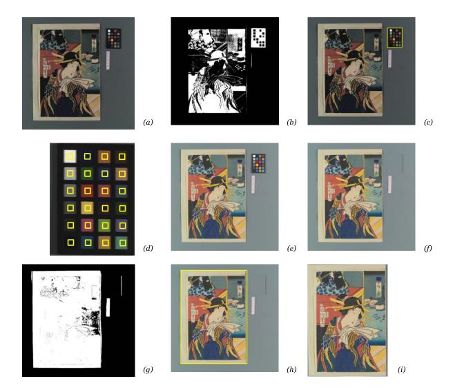
Figure 2: Automatic extraction of the colour chart and a Nishiki-e image: (a) original image; (b) binary image for detection of the colour chart; (c) detected position of the chart; (d) detection of every colour chip in the chart; (e) colour-corrected image; (f) image that the chart is masked; (g) binary image for detection of a Nishiki-e image; (h) detected position of the Nishiki-e image and (i) extracted Nishiki-e image.
