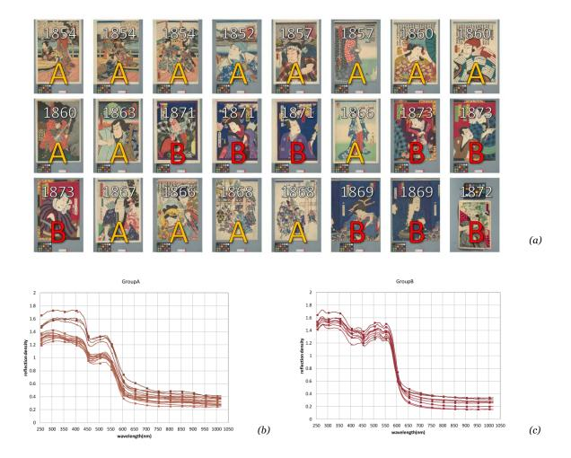
Figure 9: Spectral reflection density of old red and new red: (a) 24 samples for spectral measurement of red and its group; (b) Spectral reflection density of Group A (old red, 1852-1868) and (c) Spectral reflection density of Group B (new red, 1869-1871).
