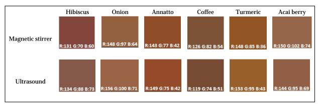
Figure 3: Photographs illustrating the influence of the type of stirring on the dyeing (extraction with water).
