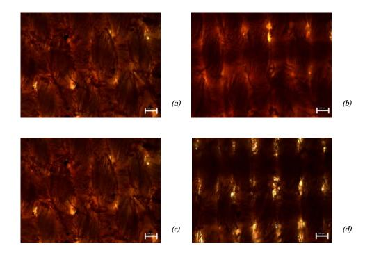
Figure 5: Optical microscopy of cotton fabric samples dyed with annatto extract: (a) water MS, (b) sodium hydroxide (MS), (c) water MS and (d) water US. Scale bar = 100 μm.
