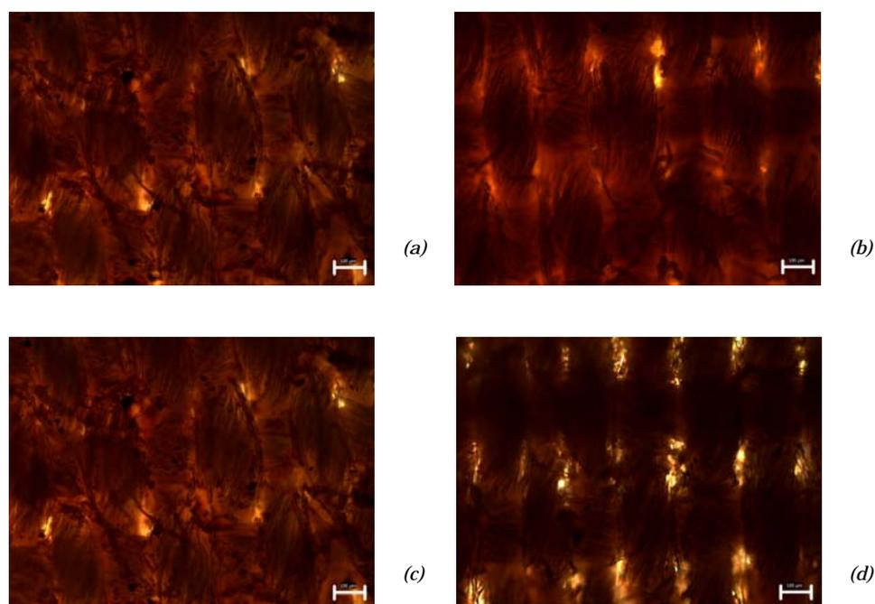
*Figure 5: Optical microscopy of cotton fabric samples dyed with annatto extract: (a) water MS, (b) sodium hydroxide (MS), (c) water MS and (d) water US. Scale bar = 100  $\mu$ m.*
