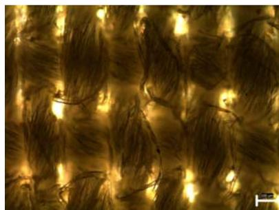
Figure 6: Optical microscopy of cotton fabric sample dyed with turmeric extract (water/ultrasound).
