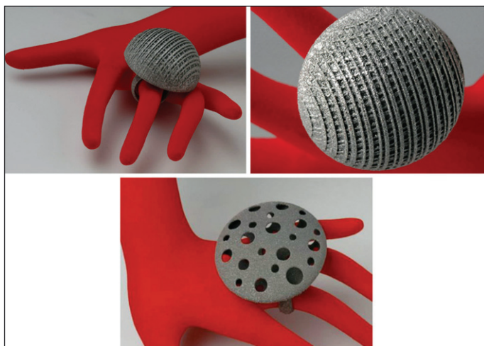
Figure 2 Production of titanium rings: hollow objects, undercuts, textures
