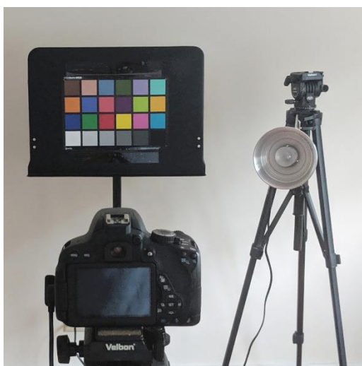
Figure 11 (left): Experimental setup for measuring lens glare.
