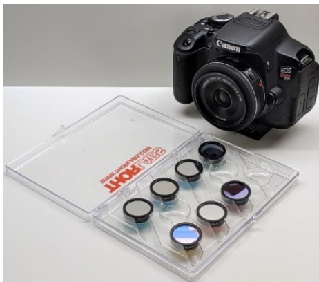
Figure 2 (left): Canon 650D camera with 40 mm prime EF lens and set of Thorlabs narrow bandpass filters.
