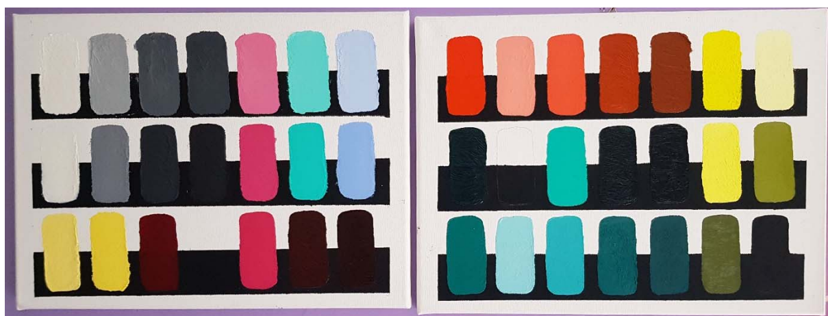
Figure 1: Photograph of 40 paint mixtures as applied on white canvas with black stripes as substrate and purple wall as background.
