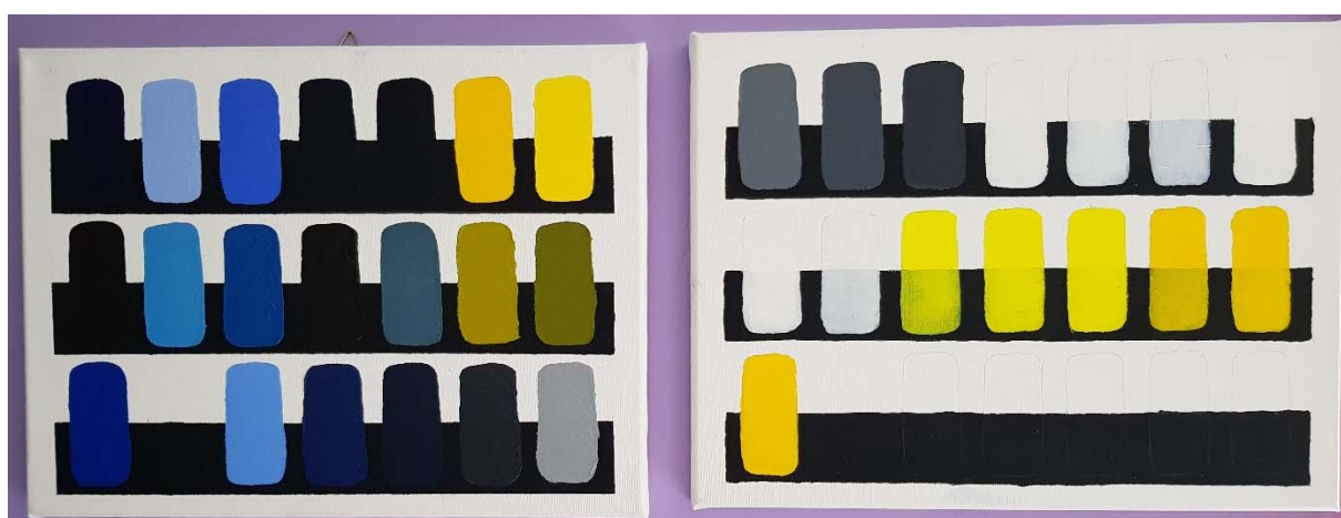
Figure 2: Photograph showing another 20 paint mixtures on the left. On the right, 15 other mixtures are shown with varying film thickness, leading to different levels of transparency.
