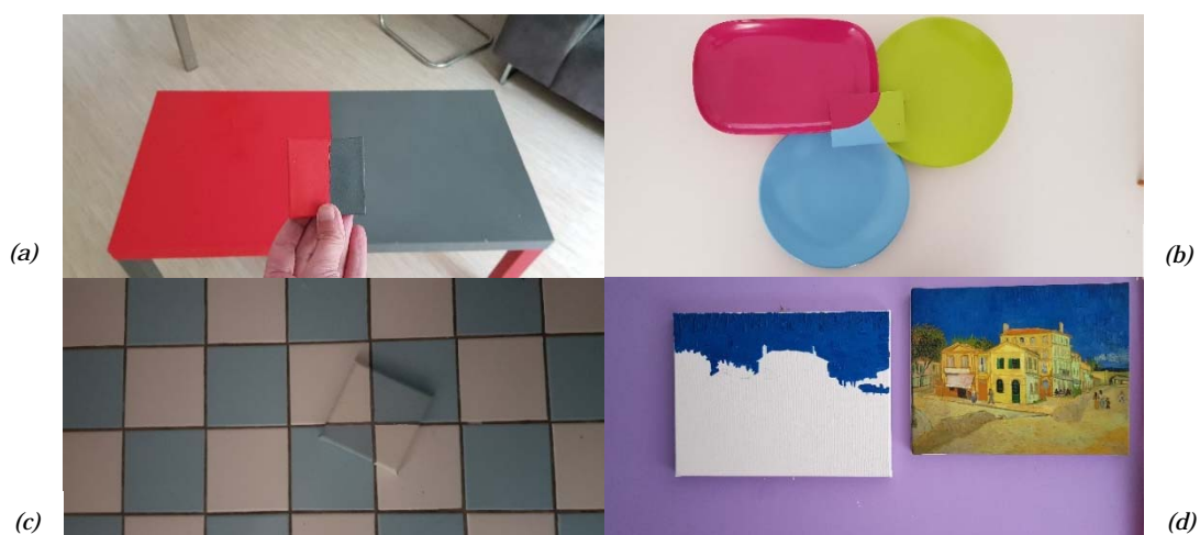
Figure 3: Photographs of dry paint mixtures. Their colours are compared to the colours of the original objects placed next to them: (a) Table grey and red samples 10 and 12, (b) Plastic plates samples 14, 15 and 16, (c) Bathroom tile samples 7, 8 and 9, (d) Blue sky in Van Gogh painting of Yellow House, samples 17-20.
