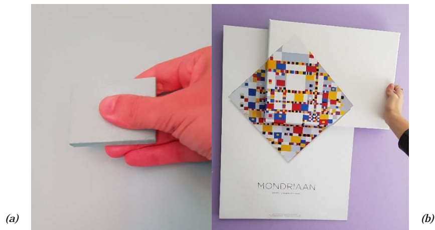
Figure 4: Photographs of dry paint mixtures. Their colours are compared to the colours of the original objects placed next to them: (a) Wall paint sample 3, (b) Various colours in Mondriaan painting Victoria Boogie Woogie, samples 21-31.
